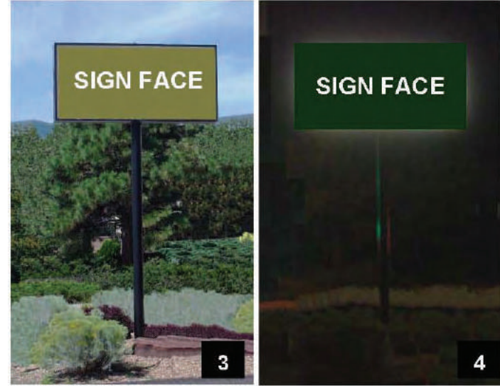
Illustration # 3 & 4 simulates night view of an internally lit box sign that only illuminates the sign message. This type of lighting is an acceptable Dark Sky practice and is an allowable use.
